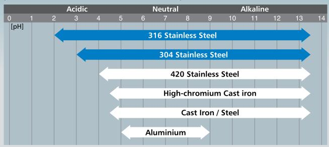
The above data is a rough indication for sulfuric acid (H2SO4) and sodium hydroxide (NaOH). Metals are affected by the type of acid/alkali, seal material, painting and abrasive environment.
